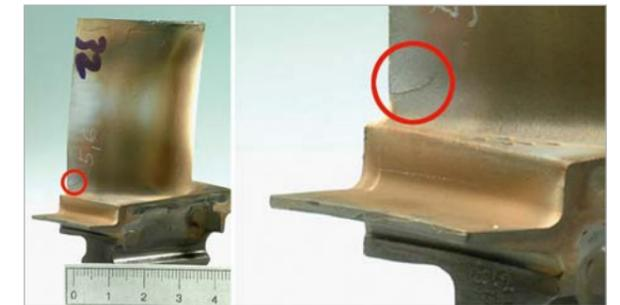
Fig. 2: Engine blade with crack on trailing edge (red circle)
