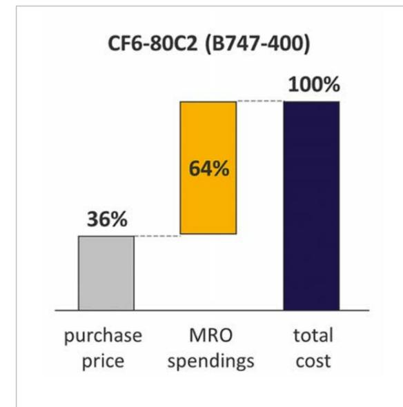
Fig. 1: Engine lifetime cost
