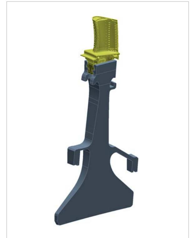
Fig. 7: FE model of the blade
