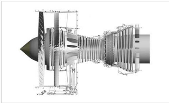
Fig. 3: Geometry of a CFM56-5C engine
