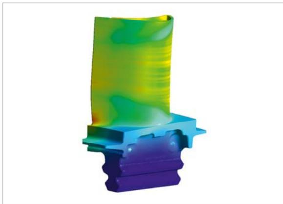
Fig. 4: Temperatures on a high-pressure turbine blade
